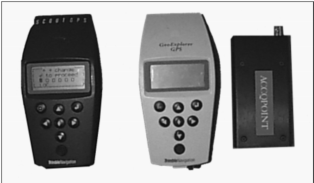
Figure 4.5 (left to right) Trimble Scout, GeoExplorer, and Accpoint FM Receiver to be used in 1996 condition survey
