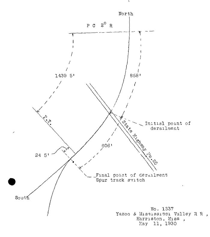
The track is laid with 90-pound rails, 39 feet in length, on treated ties, single-spiked, tie-plated, and ballasted with gravel. The track is well maintained. Under the rules, the maximum permissible speed for a passenger train with a passenger engine is 55 riles per hour.
