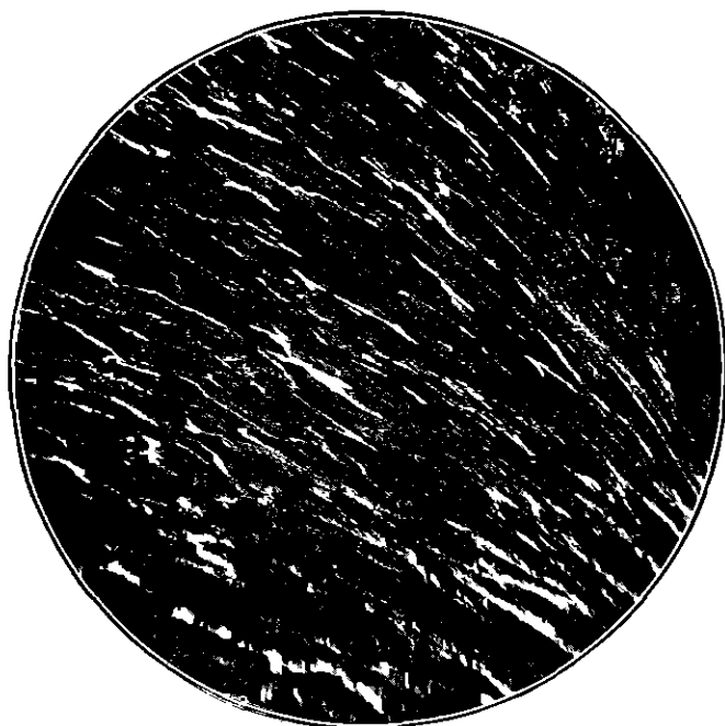
FIG. 5.--Photomicrograph of metal upper corner of head gauge side. Flattening of the grains and flow of metal at corner acted upon by the flange of the wheels. Transverse section. Magnification 100 diameters.
