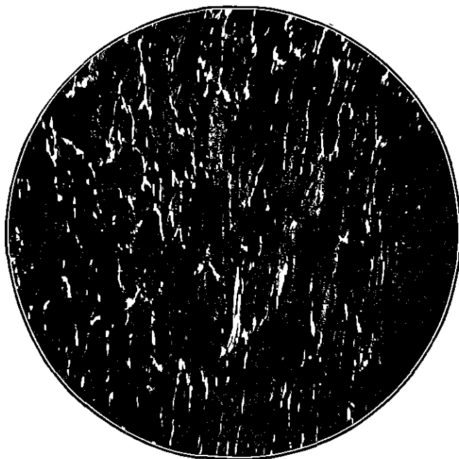
FIG. 3- Photomicrograph of metal of rail at lower corner of the head on same element as origin of fracture. Showing flattening of the grains of the steel and flow of the metal. Transverse section, magnification 100 diameters.
