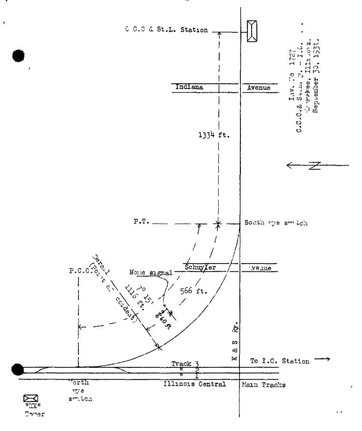
The grade for northbound trains is 0.31 per cent descending from the station to the point of accident. The track is laid with 105-pound rails, 39 feet in length, with an average of 24 ties to the rail-length, fully tie-plated, ballasted with washed gravel to a depth of from 6 to 8 inches, and is well maintained.
