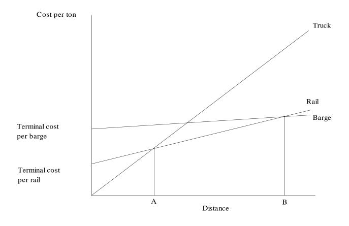
At distances less than A, truck has a cost advantage. Between A and B, rail has a cost advantage. Beyond B, barge has a cost advantage.
