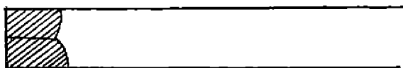
FIGURE 2—Sketch showing typical lines of rupture of crescent shaped base fractures. Shaded portion missing in this derailment.
