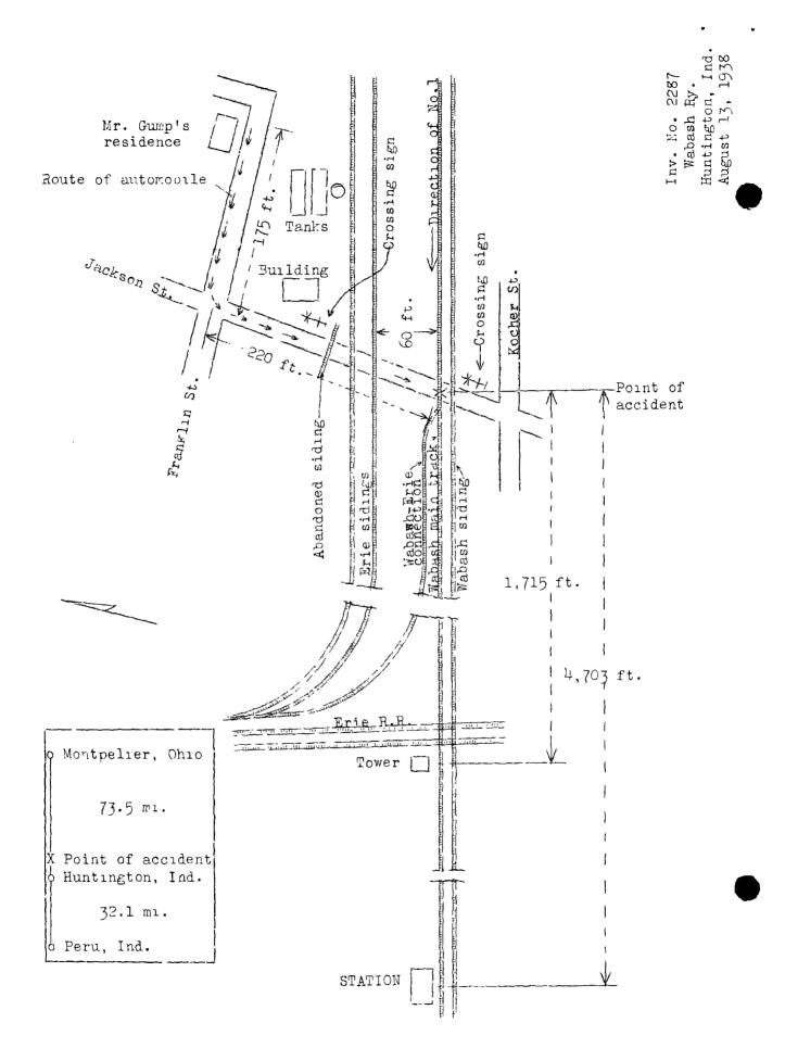
The view of an approaching west-bound train had by the driver of a south-bound vehicle is obstructed by a building and some storage tanks until reaching a point 120 feet from the main track where it is unohstructed for a distance of 760 feet; when 80 feet from the main track a clear view can be had for a distance of three-fourths mile and when 35 feet from the track the view is unobstructed. A row of telegraph poles is located 37 feet north of the main track.
