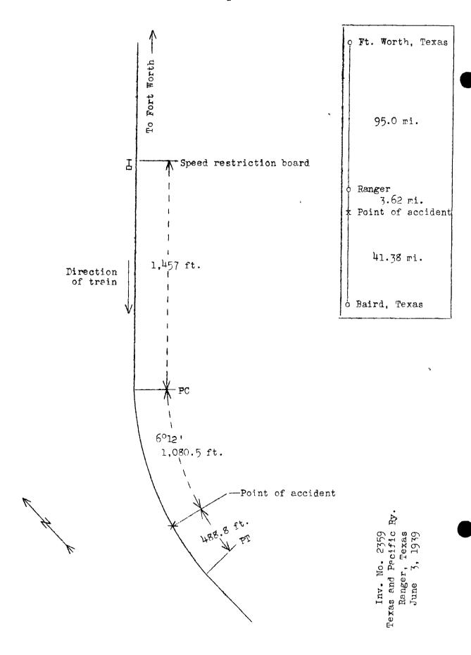
construction. This train departed from Ranger, the last open office and 3.62 miles east of the point of accident, at 11:12 a.m., according to the train sheet, 7 minutes late, and after entering the curve involved a distance of approximately 1,080 feet it was derailed while traveling at a speed variously estimated to have been between 50 and 70 miles per hour.
