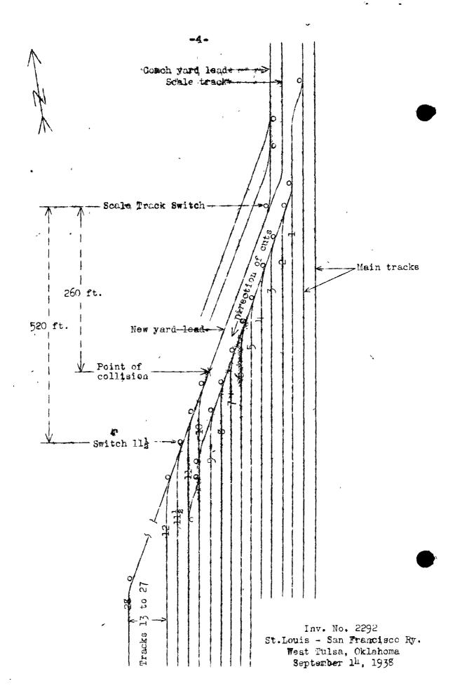
proceeded on the New Yard lead extension of the Coach Yard lead a distance of approximately 520 feet to the switch leading to track ll where it stopped to permit the proper lining of that switch. While standing at that point it was struck by a cut of cars being shoved by engine 3804.
