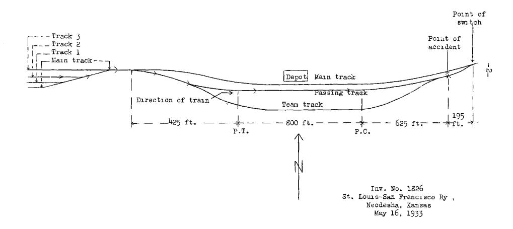
The engine, tender, and the forward truck of the first car were derailed, the engine stopping on its right side with the forward end 112 feet east of the derail, while the tender and first car remained upright. The engine was badly damaged and the tender sustained slight damage. The employees injured were the fireman and head brakeman.
