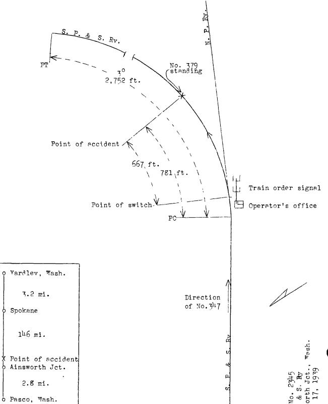
position of this switch is for a movement on the S.P.& S. track. This switch is manually operated by the operator at the junction. The operator's office is a one-story building with the door on the east side and is located about 10 feet west of the switch.
