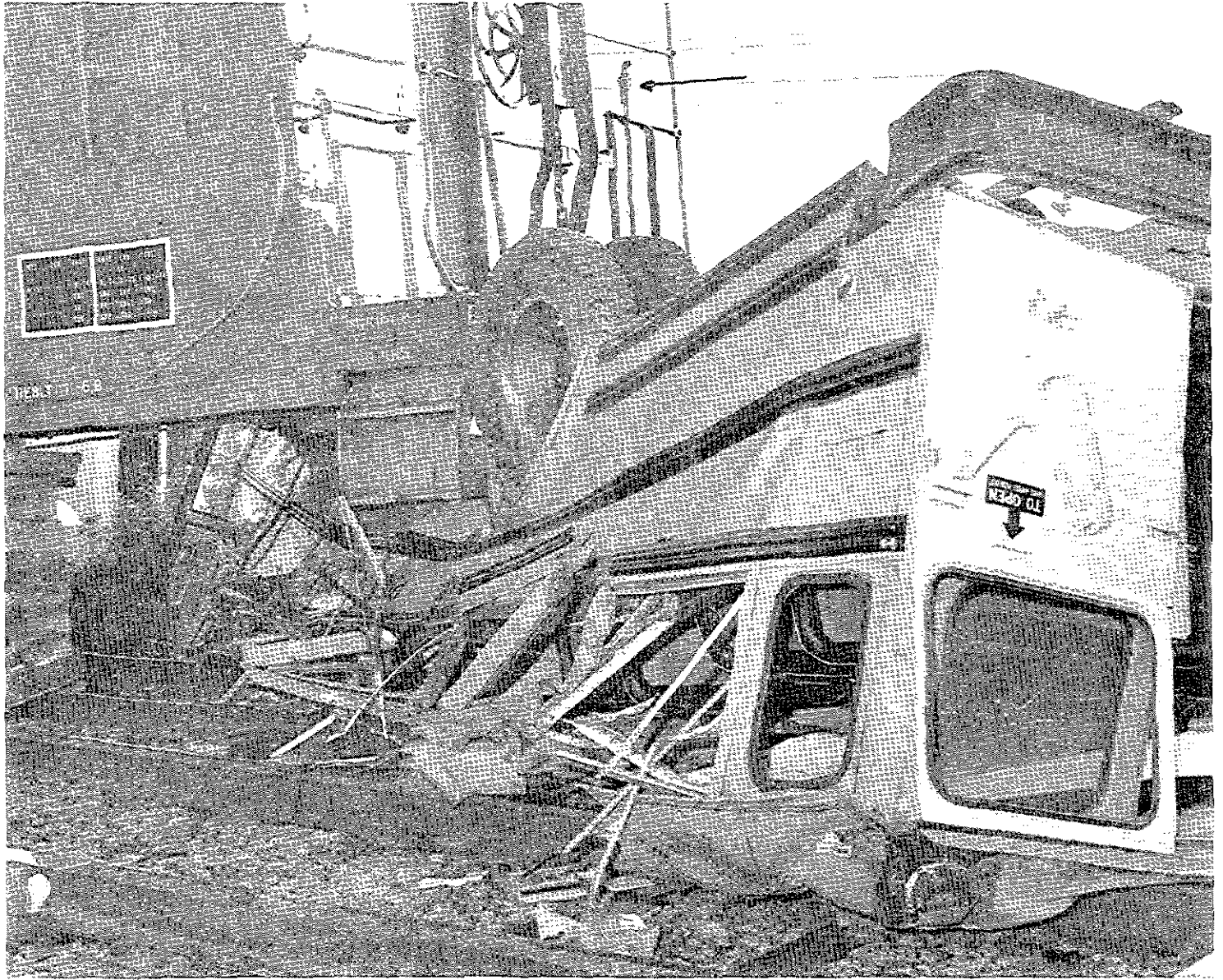
Figure A-1. Bus and caboose in final position. Note (arrow) airbrake valve.
