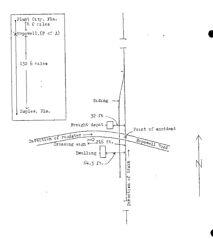
Inv. No 1785 Seaboard Air Line Ry , Hopewell, Florida Sept 21, 1932 crossing. The highway consists of a 16-foot hard-surfaced road with 5-foot dirt shoulders, and was in condition for the movement of traffic at high speed.
