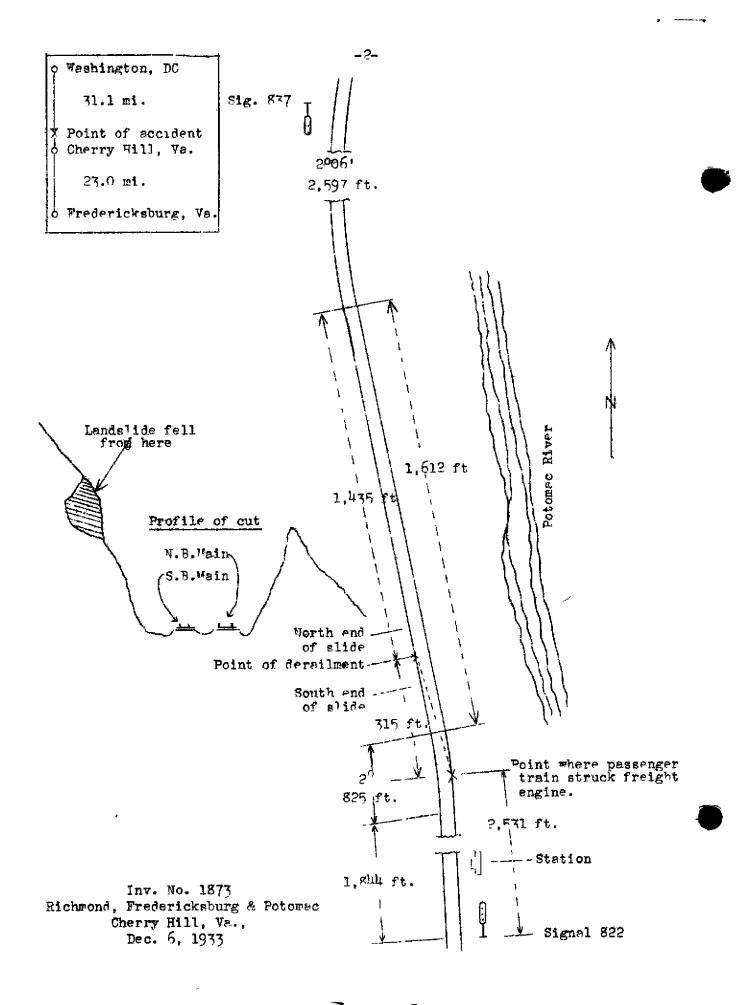
each side of the tracks between the ends of the ties and the slopes to accommodate movement of loose material or raveling; the faces of the banks are precipitous.
