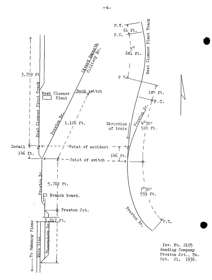
tie to engage the movable portion of the derail when it was off the rail, in order to prevent it from rising out of this position.
