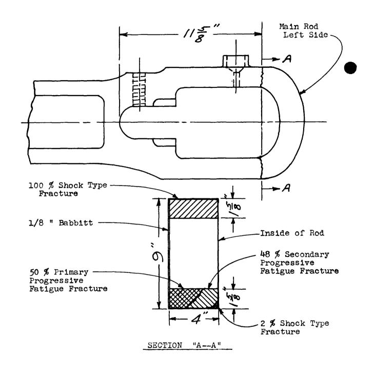
SKETCH OF FAILED FRONT END OF MAIN ROD READING COMPANY LOCOMOTIVE 130
