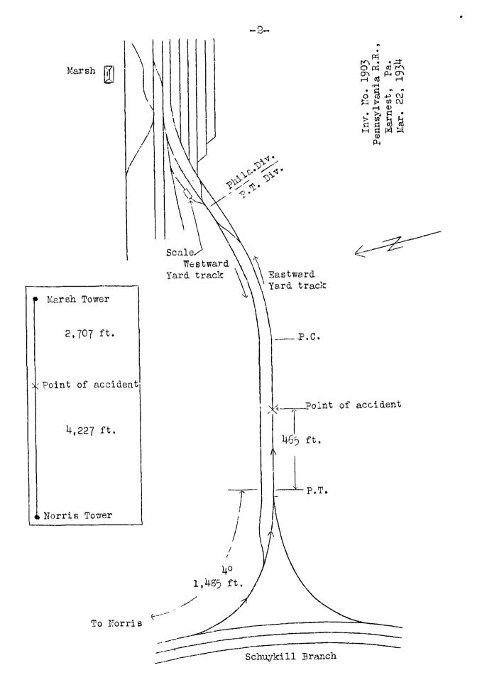
Marsh yard while passing through cross-over switches, the driving wheels of the engine commenced to slip and they continued to slip until the train stalled; slack had been taken several times in an effort to start the train when the rear end was struck by Extra 280.
