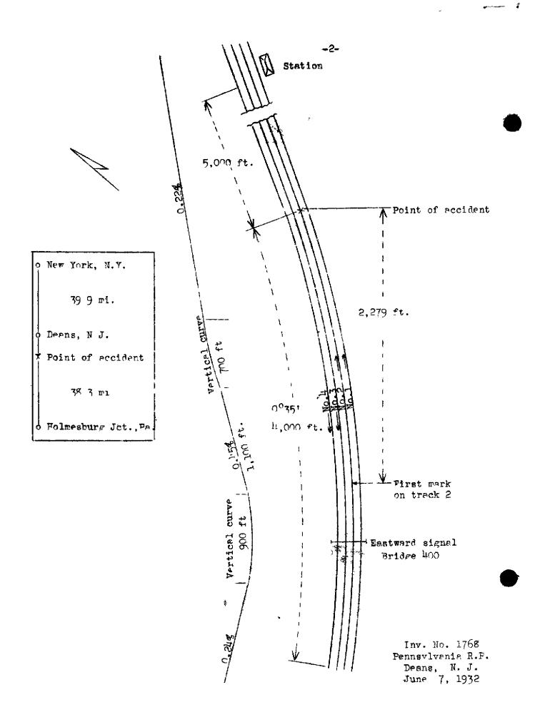
The tracks are load with 130-pound rails, 39 feet in length, with an average of 22 treated ties to the raillength, fully tic-plated, and ballasted with stone to a depth of about 24 inches. At the point of accident the track is constructed on an embankment of stone and earth about 18 feet in height, which is in good condition. The
