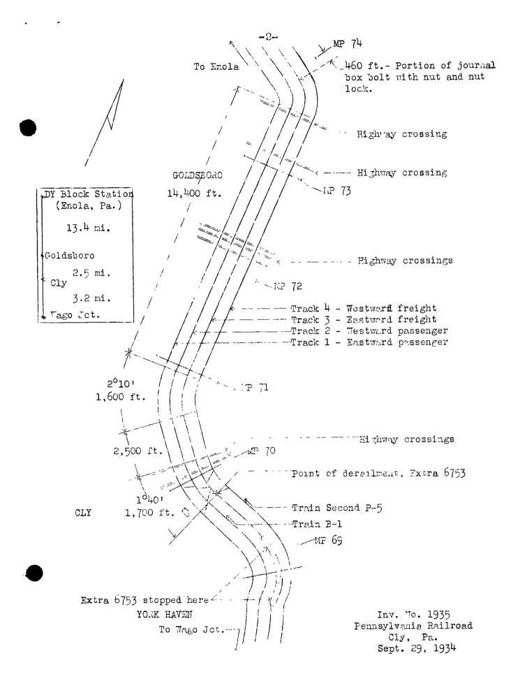
Track 3 is laid with 130-pound rails, 33 feet in length, with 18 treated ties to the rail length, fully tieplated, ballasted with trap rock, and is maintained in good condition. The maximum authorized speed for freight trains on all tracks is 40 miles per hour.
