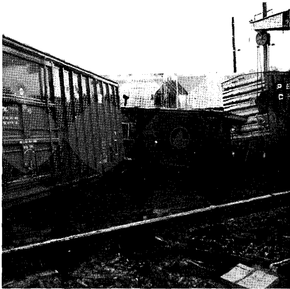
Figure 3. Derailed Penn Central boxcars in contact with B&O caboose.
