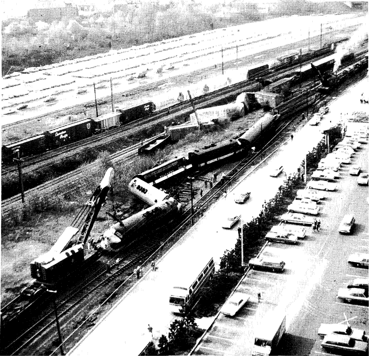
Figure 2. Overview of accident site, showing derailed freight and passenger trains.
