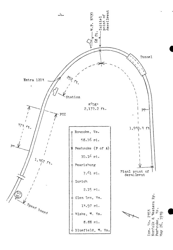
In this vicinity the track parallels New River, is laid on a side-hill cut, and passes through a stone arch tunnel 290 feet in length, the west portal of which is located 319.7 feet east of the initial point of derailment. Guard rails are laid the entire length of the tunnel.
