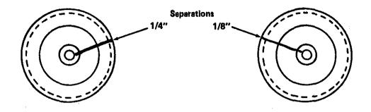
Figure 2. Broken wheels from the December 12, 1978 derailments.
