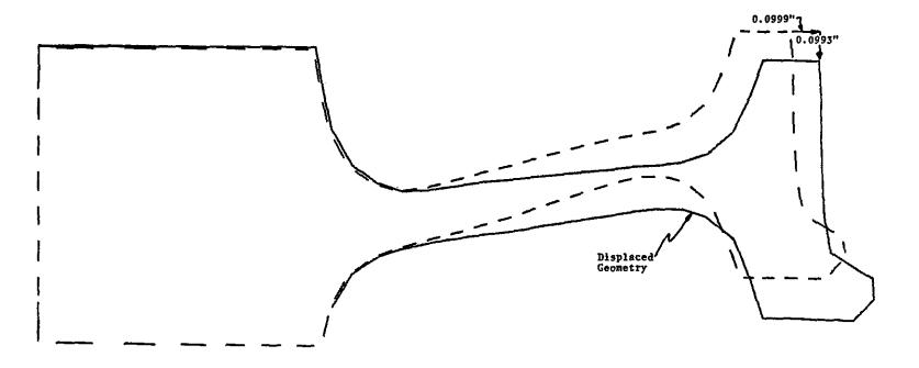
K-3 HEAVY HANDBRAKE DRAGGING DISPLACEMENTS
