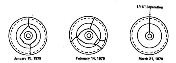
Figure 3. Broken wheels from three subsequent derailments.
