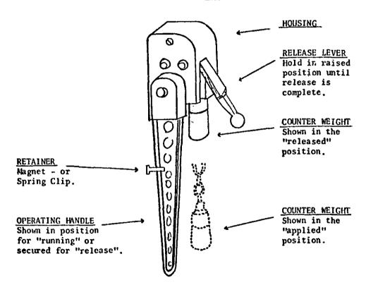
Figure 4. Peacock Handbrake Used on NYCTA Subway Cars.
