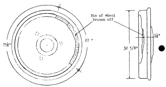
the wear was insufficient to condemn and remove the wheel. None of the broken portions of either wheel were found, due to the heavy fall of snow at the time of the accident, and to the fact that the track was badly torn up.
