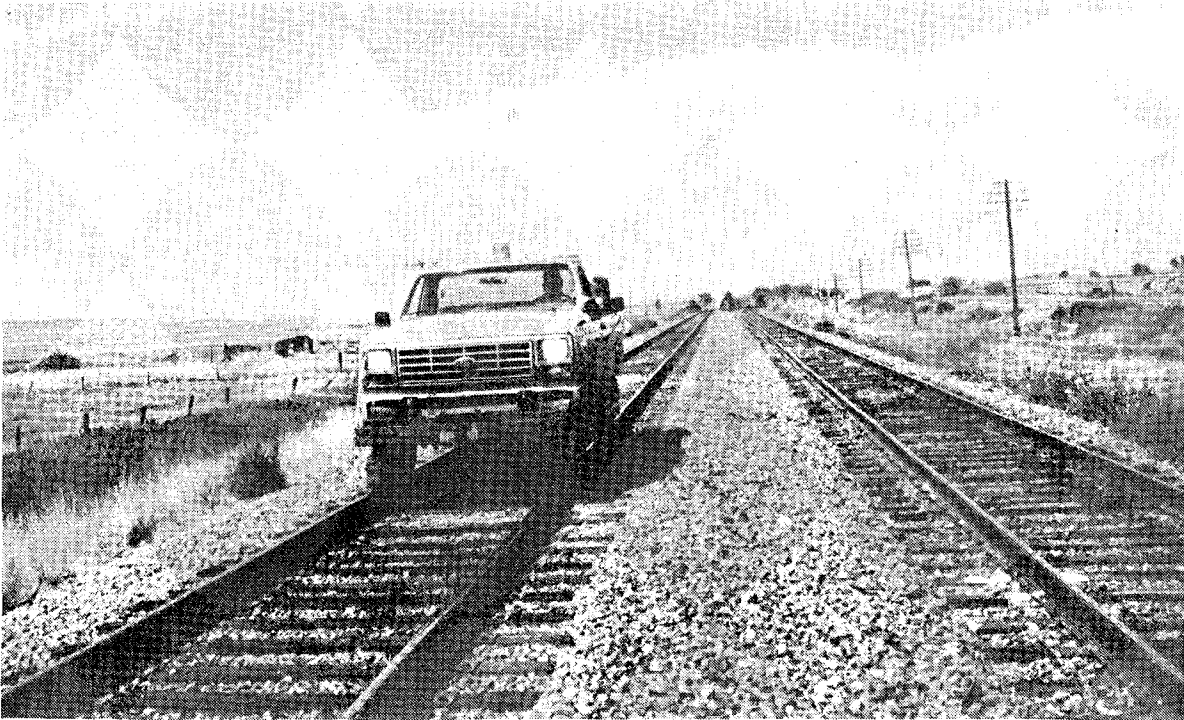
Figure 1.--Track inspector in high-rail vehicle near mp 317
