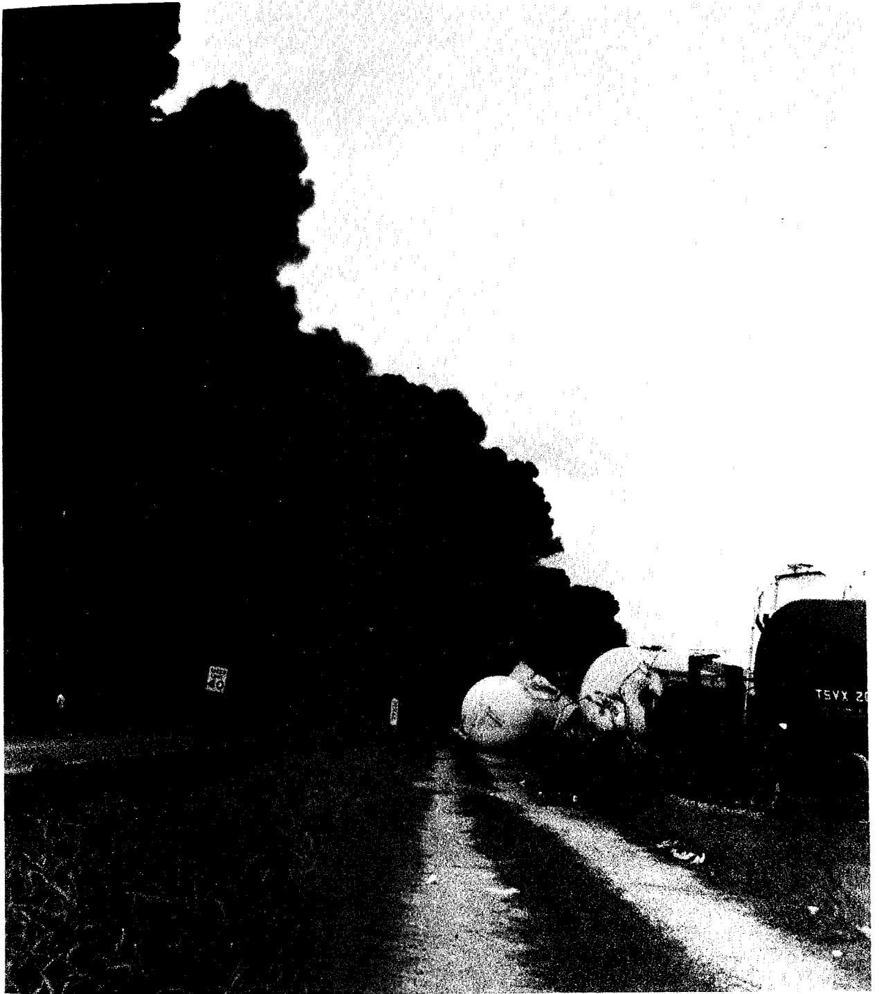
Figure 3 - View from the west side of track, south of the general wreckage prior to 2:30 p.m. on October 19, 1971. Tank car to extreme left is ESMX 4803. Car lettering and position of body bolster indicates car is inverted. Frost line indicates liquid level of contents.
