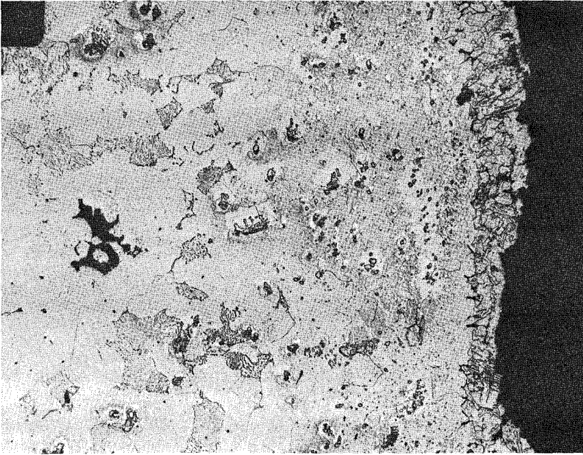
Figure 10. Typical surface along the side of the lockarm showing excessive decarburization that formed a ferritic skin on the casting surface and underlying rum of pearlite. X200 nital etched
