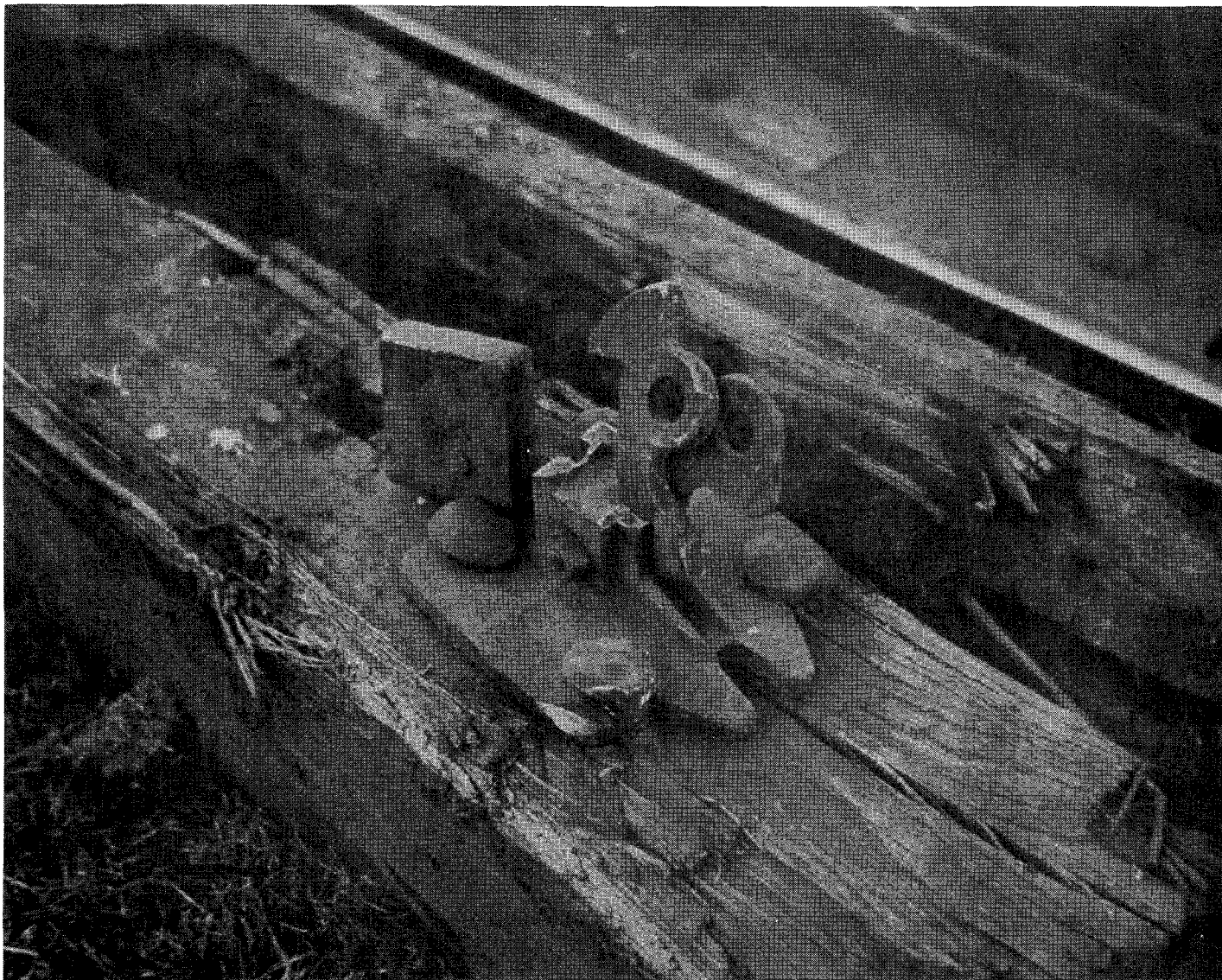
Figure 5. North foot latch of the switch stand for the north house-track switch after the accident.
