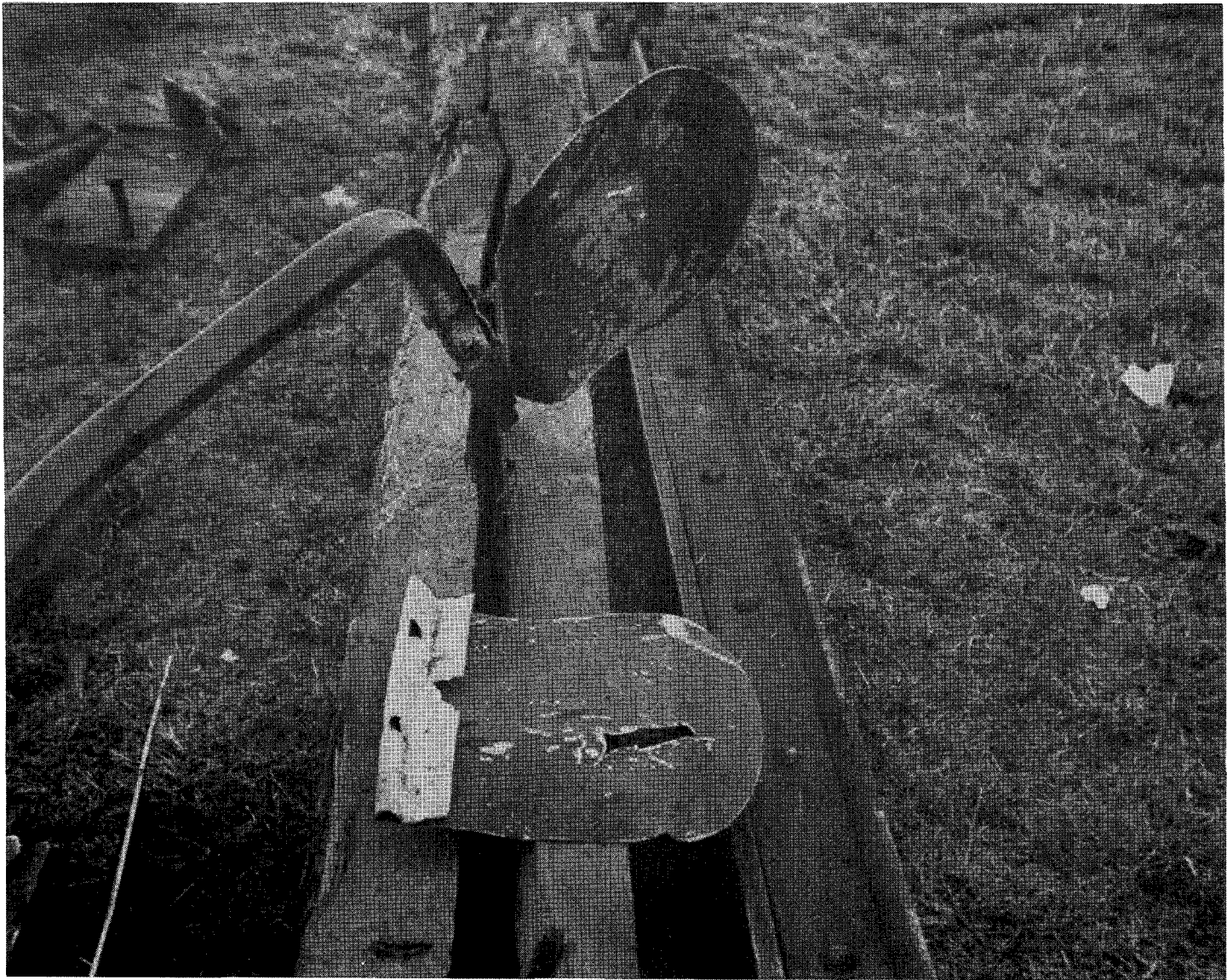
Figure 3. Switch-stand target of the north house track switch after the accident.
