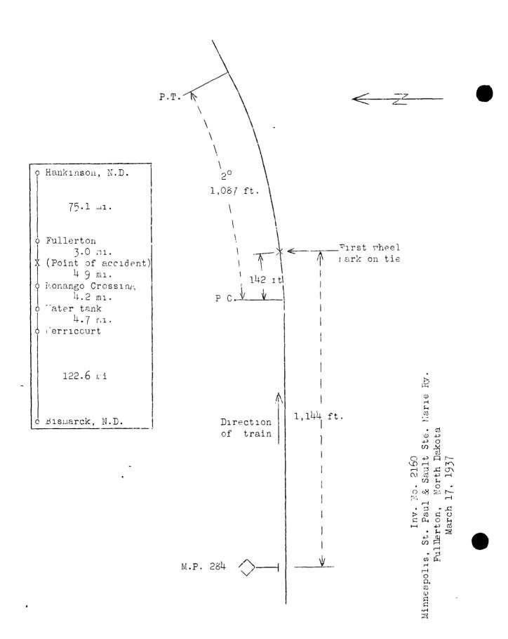
stopped for water at a point 4.7 miles beyond, stopped at Monango, 4.2 miles farther on, to let off a passenger, and on reaching a point about 4.9 miles beyond Monango was derailed while traveling at a speed estimated to have been about 25 or 30 miles per hour.
