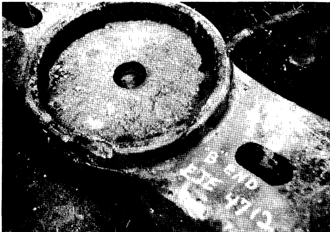
Figure 10.--Center plate of trailing truck bolster, gondola EJ&E 4712, with lower remnant of center pin lodged in the bolster.
