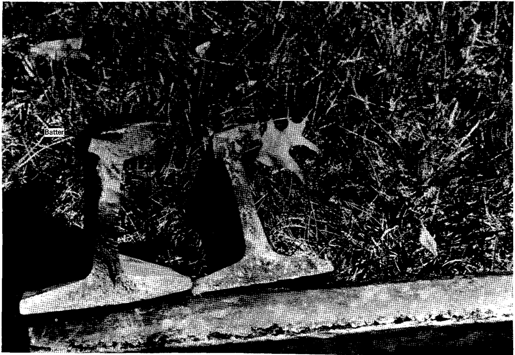
Figure 6.—Batter marks on section of broken rail.
