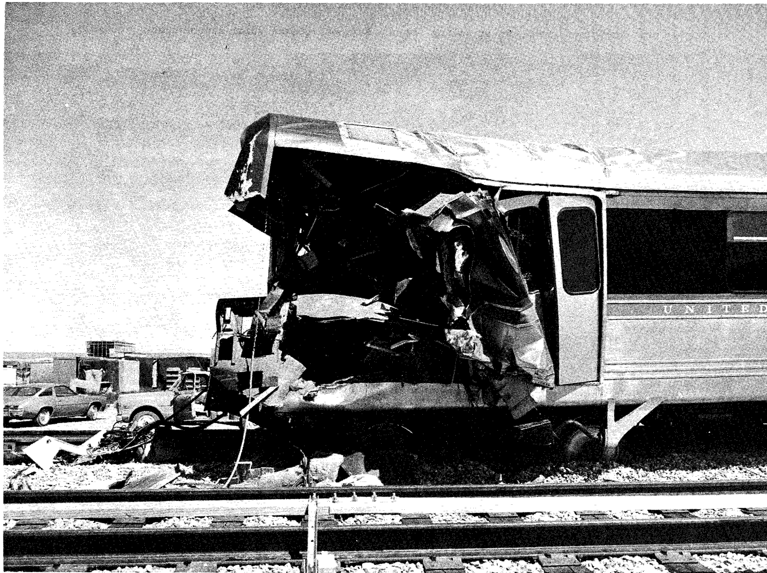
Figure 3. Damage to the west side of the SOAC .
