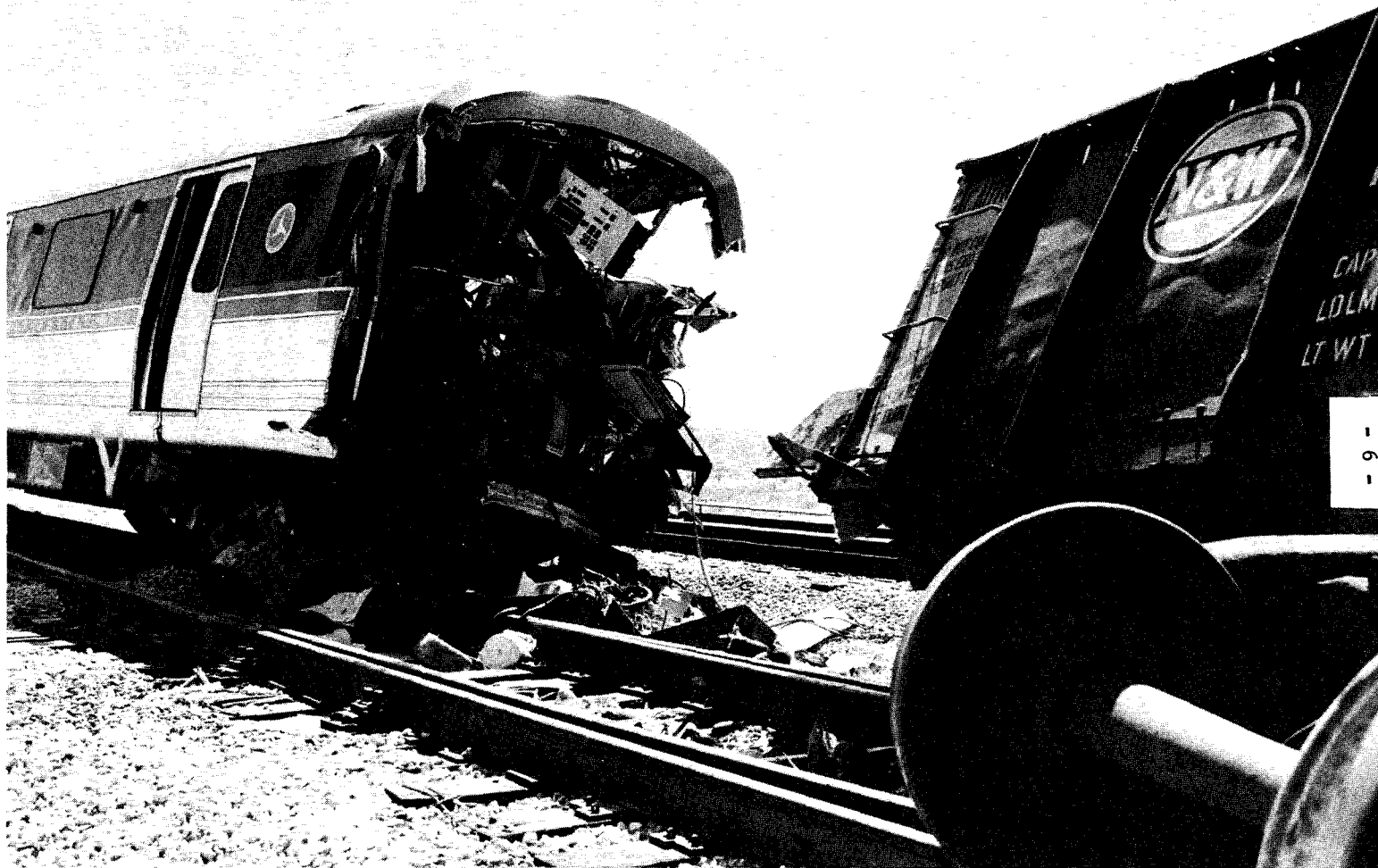
Figure 2. Demolished operating compartment and the east side of the SOAC car. Derailed gondola car is at the right.
