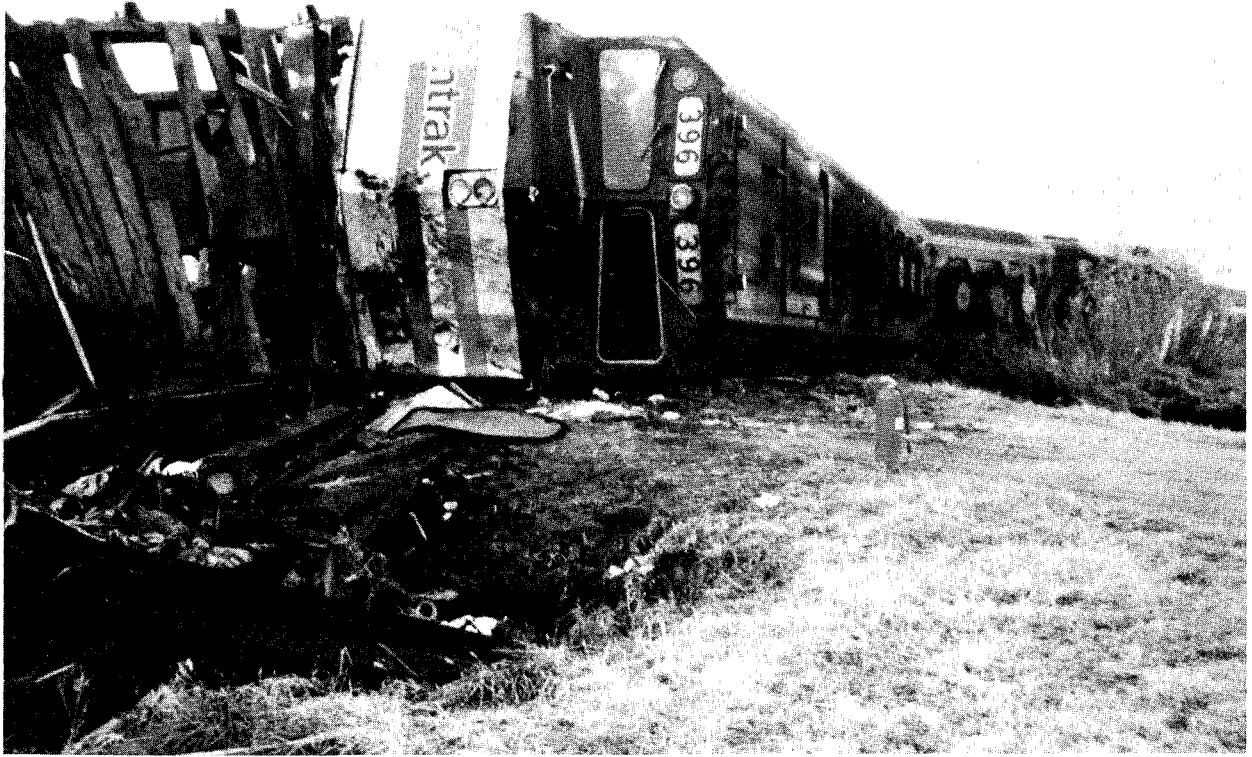
Figure 7 --Locomotive of train 6 after the collision
