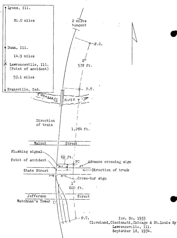
farther south. From midnight to 6 a.m., within which period this accident occurred, no watchman is on duty and the flashing light signals are not in service. There is an advance railroad-warning sign of the reflector type on a pole on the north side of State Street located about 250 feet east of the crossing; also a crossbar sign on the south side of State Street about 20 feet east of the track. There was no sign to indicate the hours during which the flashing-light signal was not in service.
