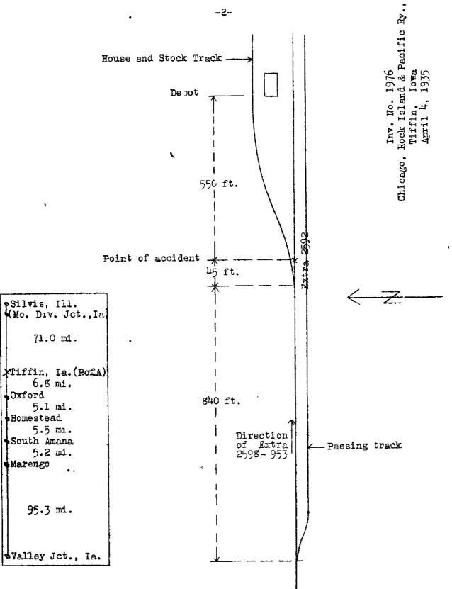
track parallels the main track on the south, the west switch being about 840 feet west of the house-track switch. The depot is located between the main track and the house track.
