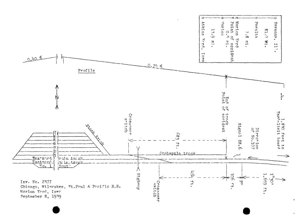
Automatic block signal 88.6 governing westward movements on the westward track is located 98 feet east of the east end of Crabapple track.
