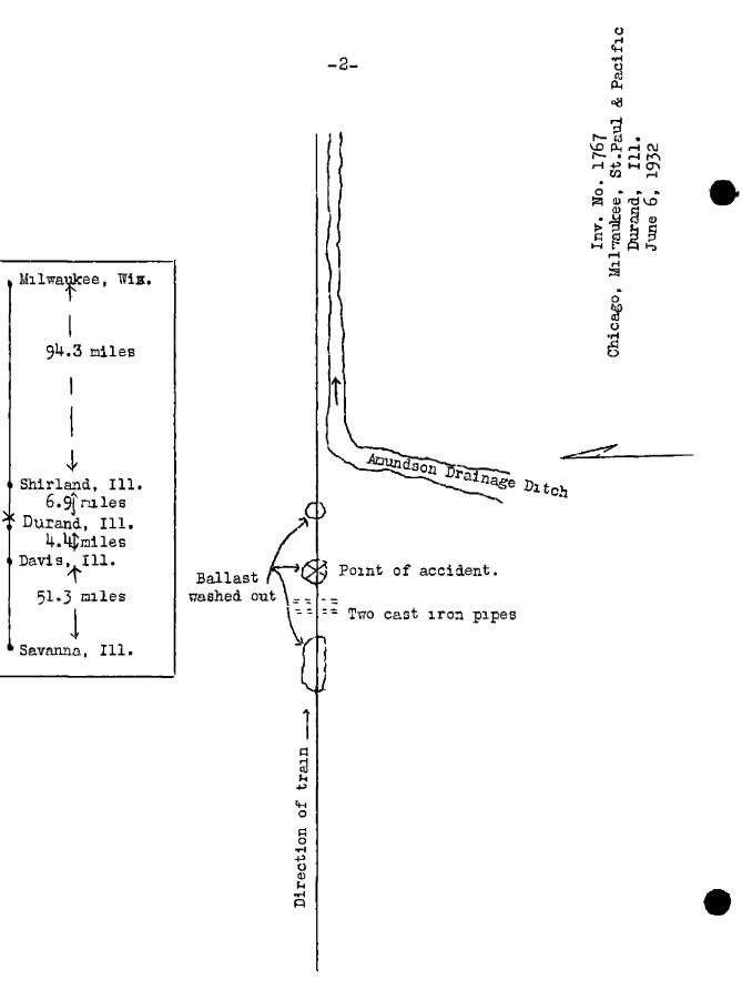
such water as drains from the west, as well as from a few hundred feet to the east, is diverted under the track from south to north through two 24-inch pipes, which were installed in 1904. The derailment occurred about 18 feet east of these pipes.
