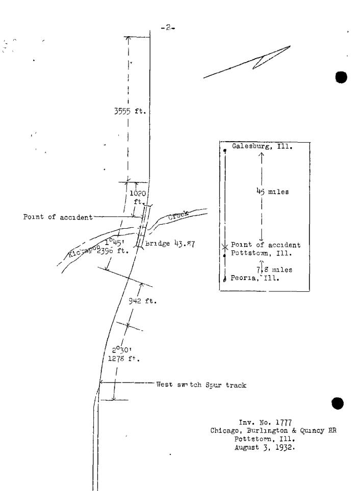
car on the team track at Pottstown, after picking up this car the train was pulled ahead a distance of approximately 1,020 feet where it was again stopped to set out a car with a hot box, and while standing at this point the rear end of the train was struck by train No. 56.
