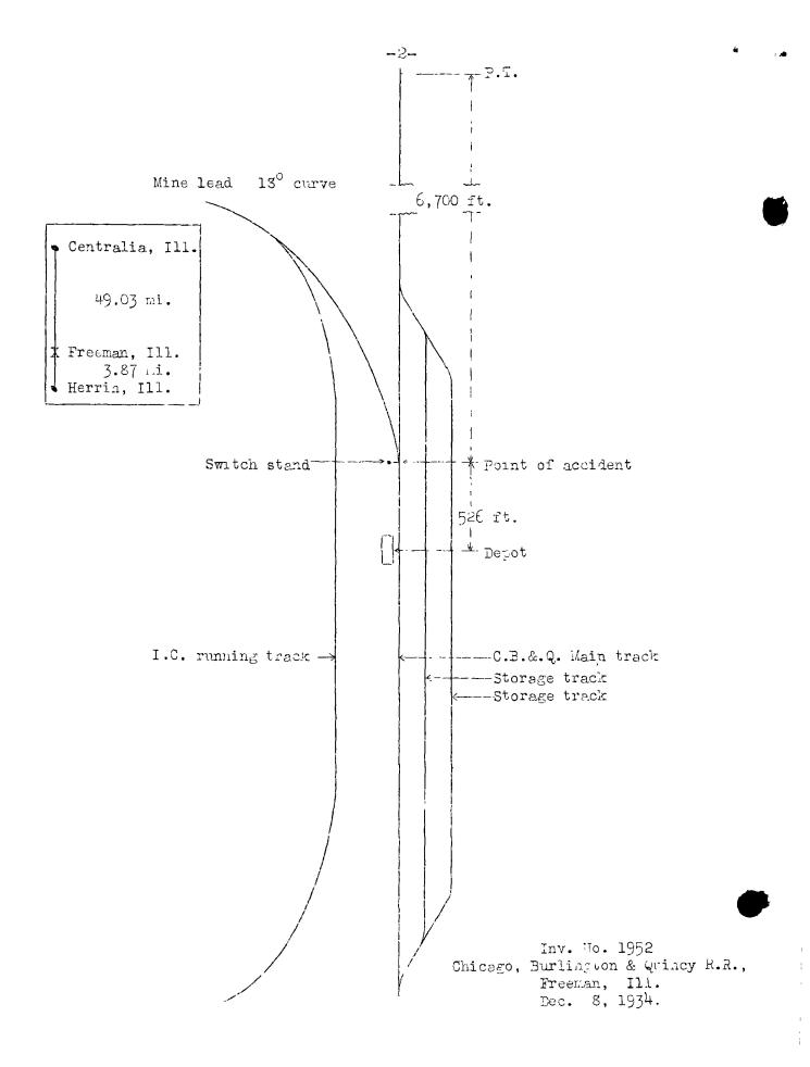
from the mine track can not be seen by the engineman of a southbound train on the main track until the caboose is close to the main track.
