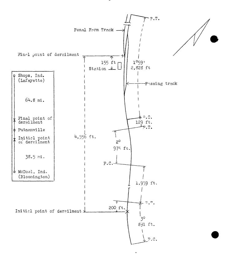
Inv. No. 2070 C. I. & L. RY. Putnamville, Ind. June 12, 1936. Permanent speed restrictions not shown in the time table are designated by speed boards. The initial point of derailment occurred within speed restricted territory of 25 miles per hour, the restriction board being located approximately 2 miles south thereof and the resume-speed board being located 175 feet north thereof, this latter board governing the territory up to and beyond the final point of accident.
