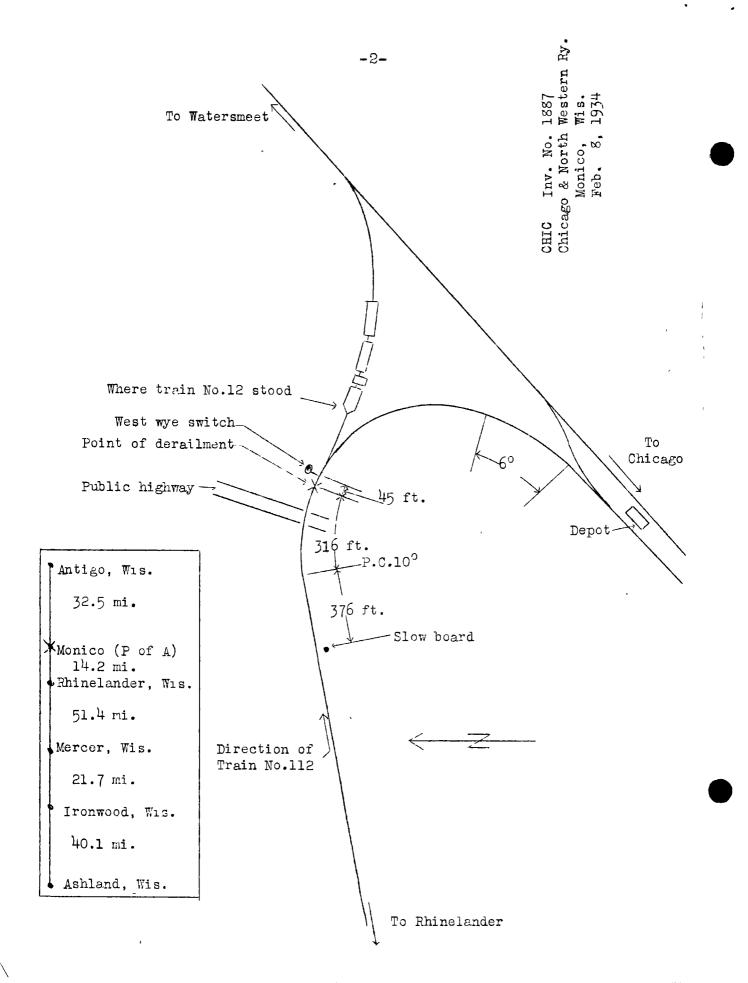
gauge varied from 4 feat  $8\frac{3}{4}$  inches to 4 feat  $9\frac{1}{4}$  inches, the track being well maintained. Under speed restrictions contained in the current time table, the maximum speed for passenger trains in the territory where this accident occurred is 55 miles per hour, and on the curve speed is limited to 25 miles per hour. There is also a slow board located on the south or engineman's side of the track at a point 375 feet west of the curve.
