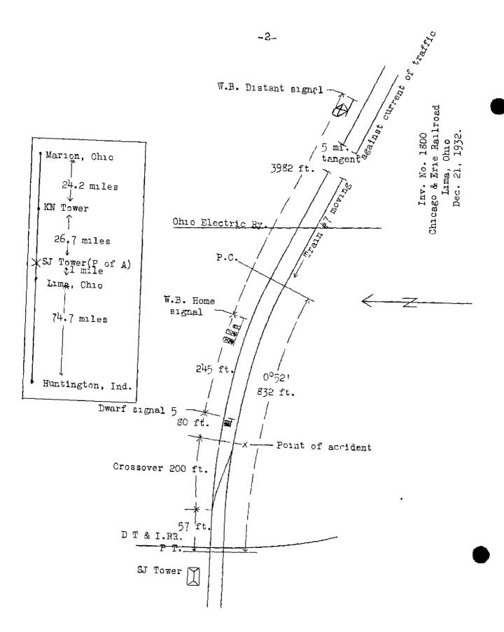
Under special instructions contained in the time-table, the speed of trains through crossovers is restricted to 10 miles per hour.
