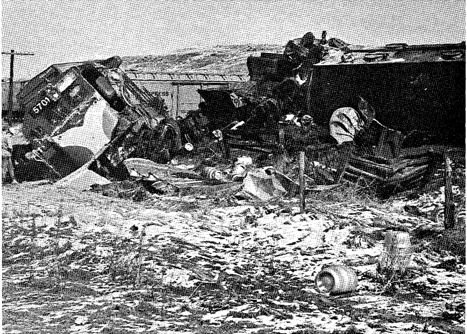
Figure 4.—Derailed unit 5701 showing location, position, and general condition after impact.
