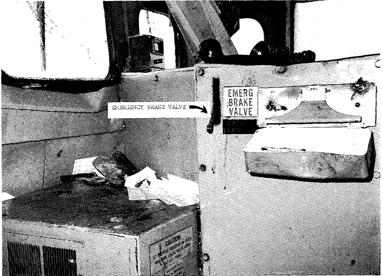
Figure 3.—Locomotive cab interior showing the emergency brake valve.
