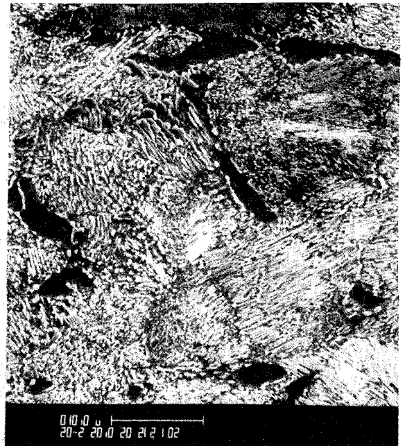
Figure 10. Comparative SEM micrographs of section B-B. Left photograph taken 0.01 inch from tread surface and is typical of area "H" Figure 9. Right photograph was taken approximately 0.5 inch from tread and is representative of microstructure to right of area "H" shown in Figure 9. X2000 nital etched.
