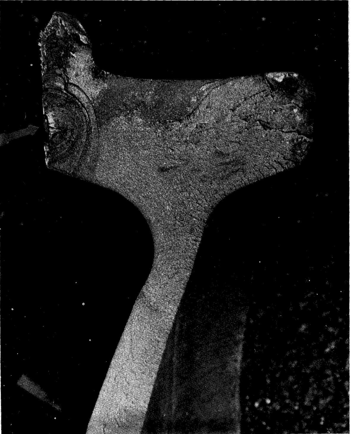
Figure 3. Cross-section of R-3 wheel from car No. 49.
