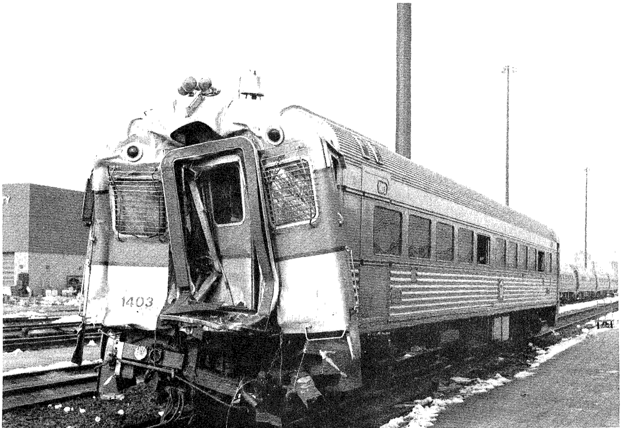
Figure 4.--Damage to the control car (1403) of train 8114.
