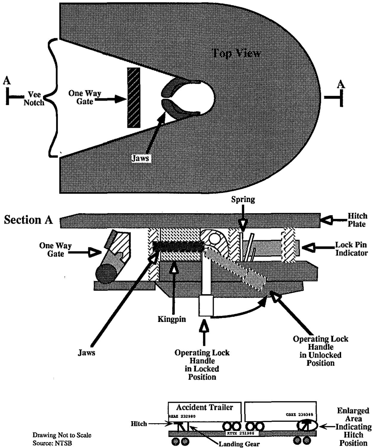
Figure 5. -- Intermodal trailer type III hitch and kingpin.
