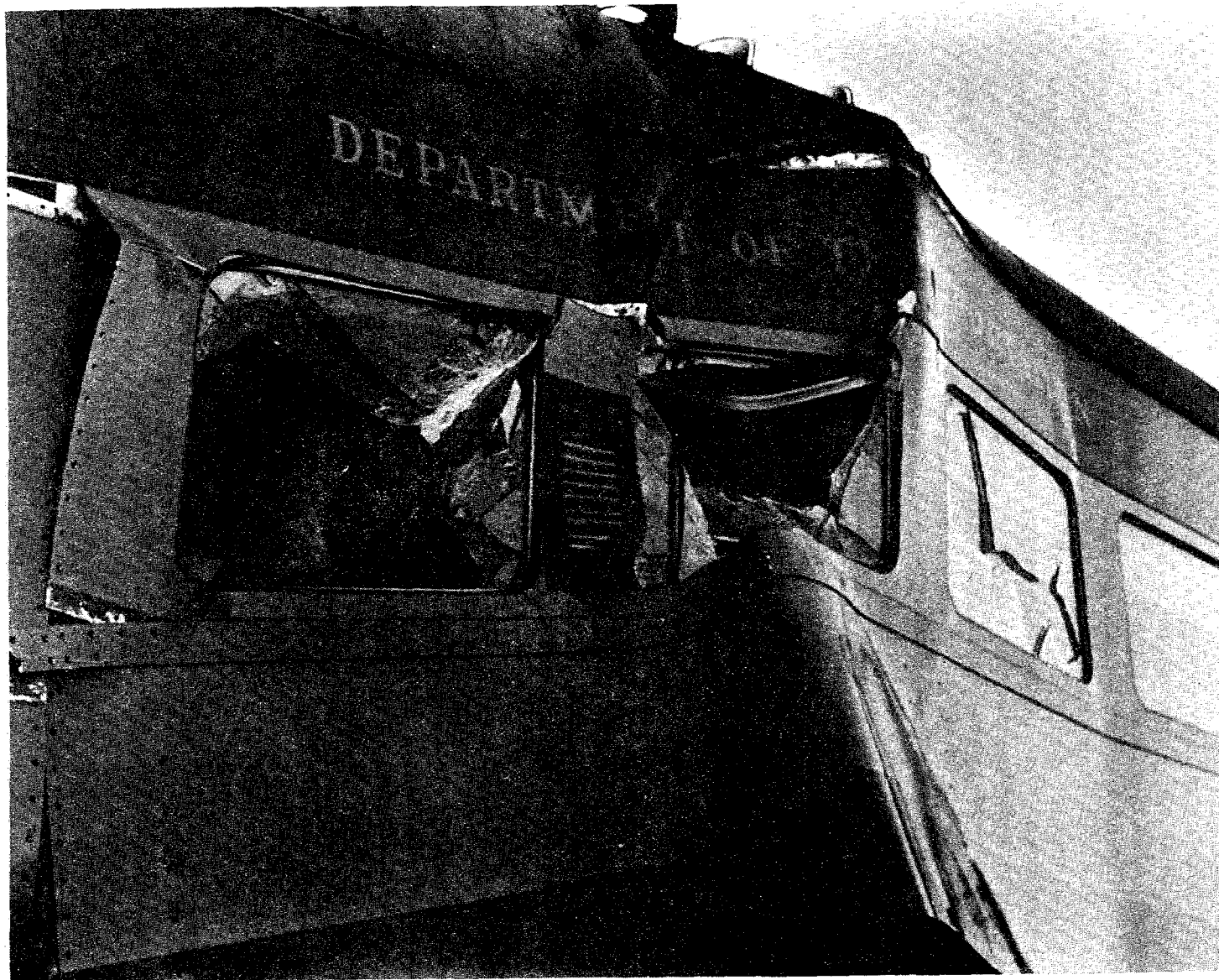
Figure 1. Damaged dome car of train No. 5.
