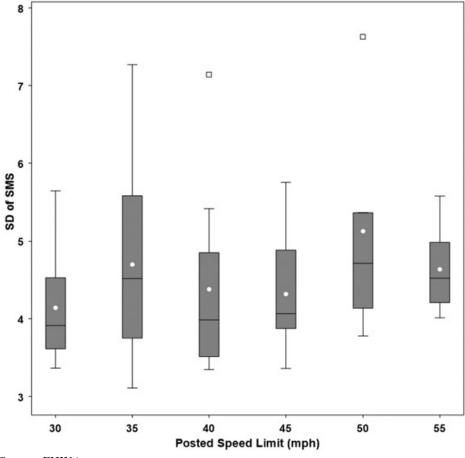
Figure 25. Graph. Box plot of SD of SMSs on 2U sites by PSL.
