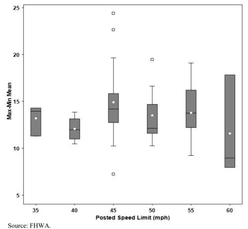
Figure 28. Graph. Box plot of the mean individual-trip maximum minus minimum speed on 4D sites by PSL.
