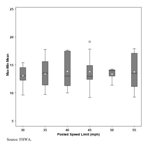
Figure 27. Graph. Box plot of the mean individual-trip maximum minus minimum speed on 2U sites by PSL.
