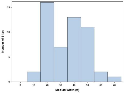
Figure 10. Histogram. Distribution of median widths for 4D arterial sites.
