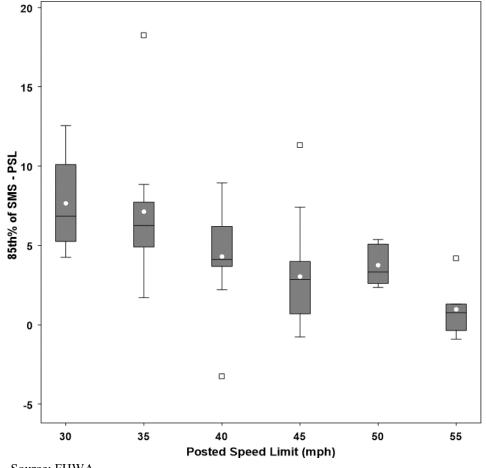
Figure 29. Graph. Box plot of the 85th percentile of SMS minus PSL on 2U sites by PSL.
