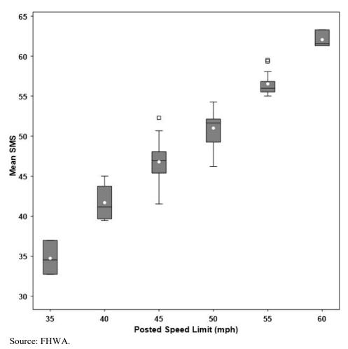
Figure 24. Graph. Box plot of mean SMSs on 4D sites by PSL.
