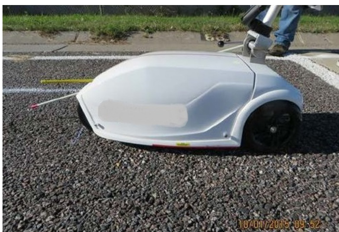
Figure 6. Photo. Walking profiler (FHWA Office of Technical Services Resource Center P&M TST 2015).
