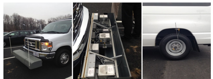
Figure 7. Photos. Components of a typical inertial profiler system (Nicks and Adams 2017).
