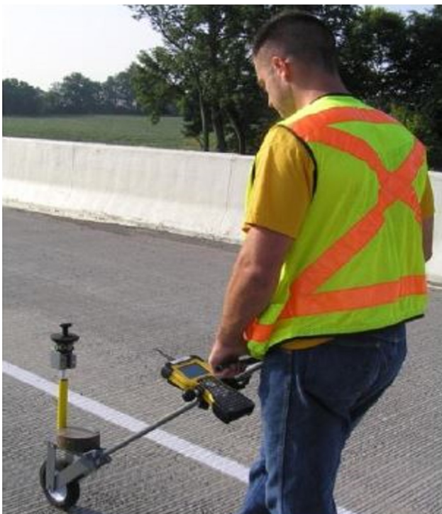
© 2011 Iowa State University of Science and Technology. A. Monowheel cart and 360-degree prism.
