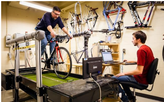
a) Vertical excitation on front wheel test on a treadmill (CYCLETIPS 2018)
