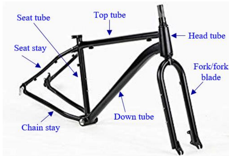
Figure 2-4. Diamond frame of a bicycle with fork
