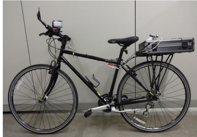
Figure 3-11. Instrumented probe bicycle (IPB) (Oh et al. 2017)
