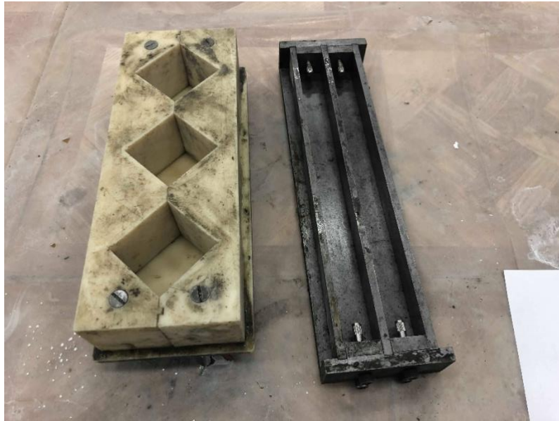
Figure 2.11: Mortar cube and bar molds
