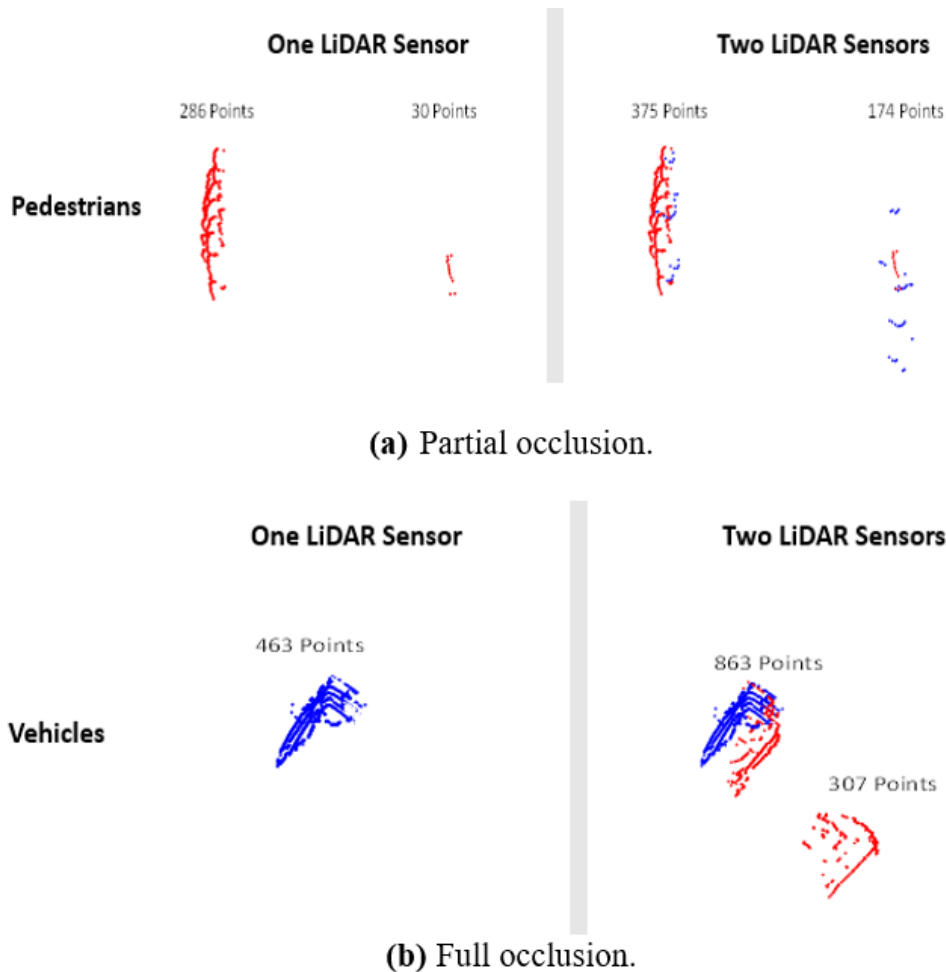
Figure 0-19 Demonstration of multiple-LiDAR overcoming occlusion
