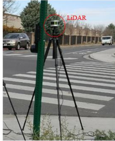
(a) Permanent installation (b) Temporary installation Figure 0-7 Different installation methods of roadside LiDAR sensors
